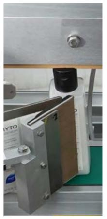
A 3-roller workstation with gate allows the application of two opposing labels placed alternately on the backing paper.
