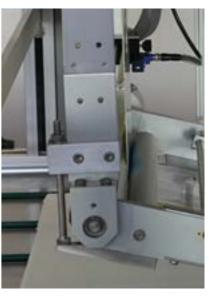
Thanks to a "stop device" the end is reset in the pre-set position after a thicker product transit.
