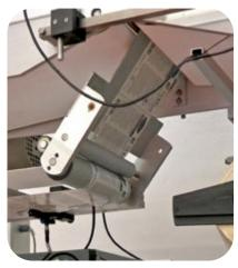
The **upper labeller** is equipped with an **adjustable long dispensing terminal for a 20 x 40 mm label** separation from the backing paper and its application on the product.
