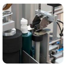
Orientation is initiated by means of a colour photocell that uses the transparent side strips of the product as a guide. The device also allows extra format change and wrap-around labelling.
